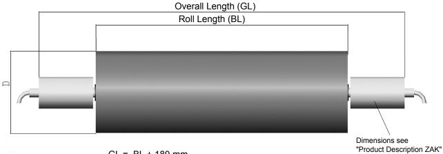
GL = BL + 180 mm axial movement (floating bearing) 174 - 183 mm
