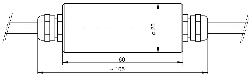
**Cable Amplifier CA-USB****Configuration and Evaluation Software**
