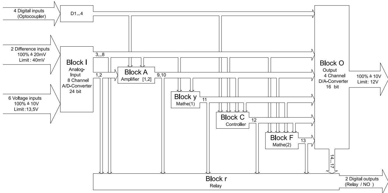
The software of the DCM is designed in blocks. These blocks are independently working functional units which can therefore be independently configured and their inputs and outputs can be assigned at will. All outputs can be visualized via the display. This simplifies fault diagnostics in customer equipment, e. g. the raw data signals of the sensor signals can be reviewed without a measuring instrument.
