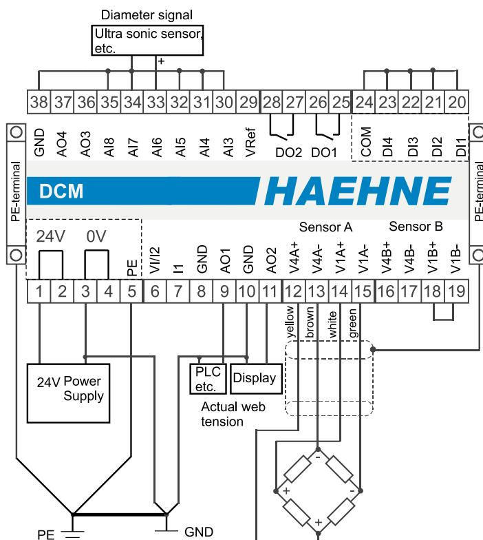
The two channel amplifier can be used for wrap angle correction on the second channel if the identical web geometry is present. For all practical purposes this is the case with a measuring roll with two sensors and separate amplification. In this case the parameter A440 is adjusted to 3.
