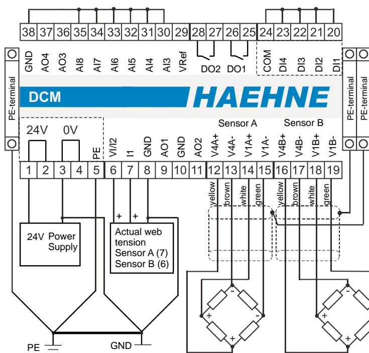
At the sensor inputs several sensors can be connected in parallel to the terminals. In this case the average is determined in analog fashion. The maximum supply current must not be exceeded.
