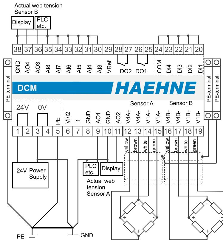
At the sensor inputs several sensors can be connected in parallel to the terminals. In this case the average is determined in analog fashion. The maximum supply current must not be exceeded.
