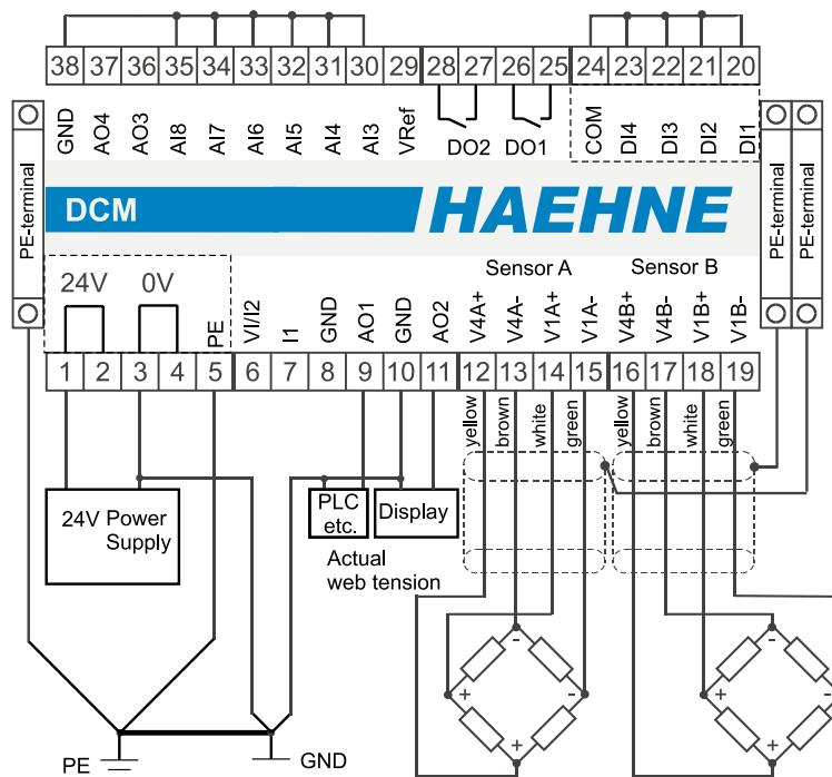
Alternatively, both sensors can be connected in parallel to terminals 12 to 15.
