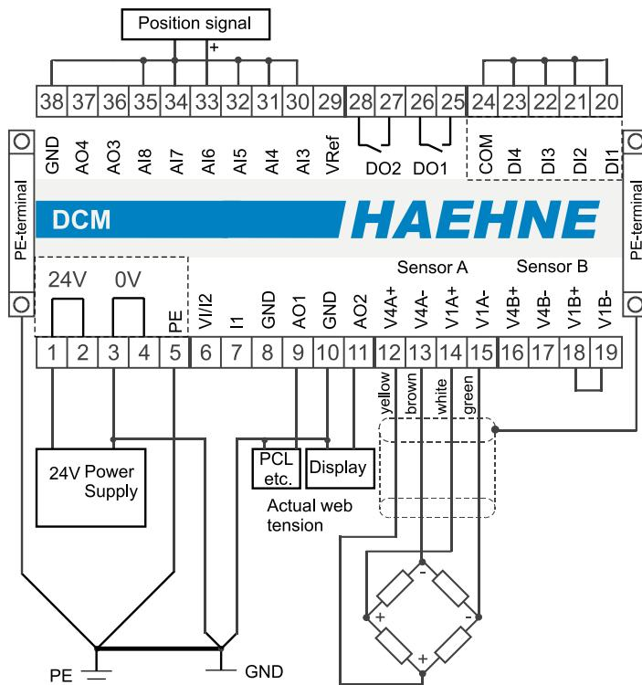
The two channel amplifier can be used for wrap angle correction on the second channel if the identical web geometry is present. For all practical purposes this is the case with a measuring the roll with two sensors and separate amplification. In this case the parameter A440 is adjusted to 3.
