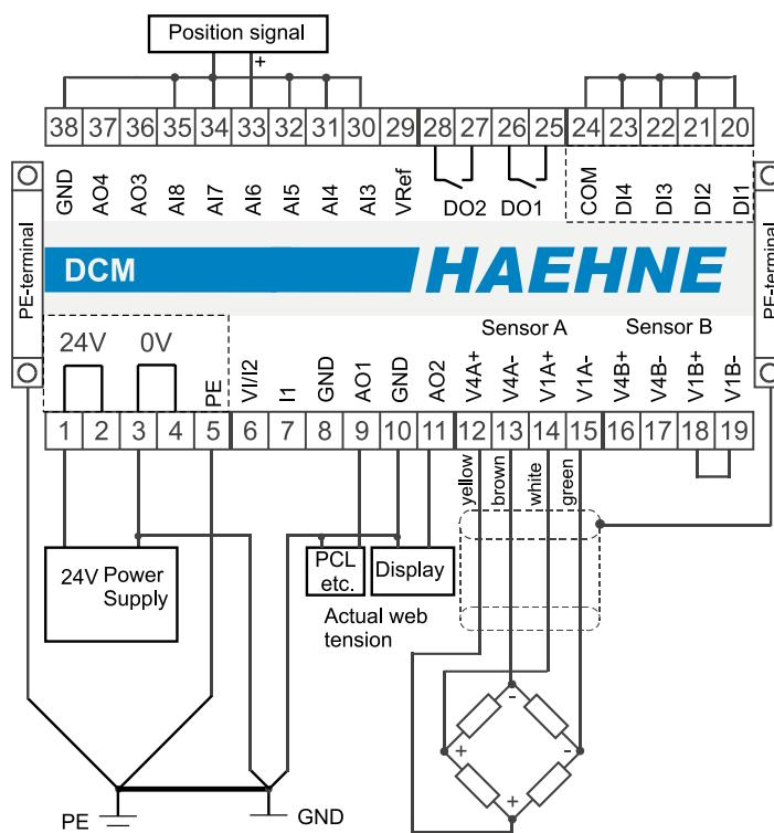
The two channel amplifier can be used for wrap angle correction on the second channel if the identical web geometry is present. For practical purposes this is the case with a measuring roll with two sensors and separate amplification. In this case the parameter A440 is adjusted to 3.
