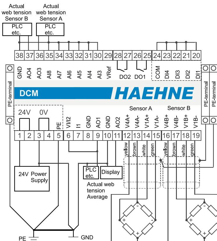
At the sensor inputs several sensors can be connected in parallel to the terminals. In this case the average is determined in analog fashion. The maximum supply current must not be exceeded.
