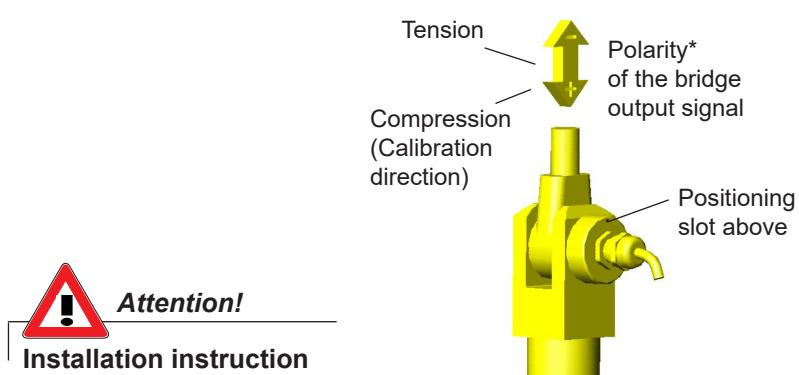
\*Align positioning slot according to action line of the measuring direction. In order to obtain reverse polarity turn the KMB by 180° (positioning slot is at the bottom).
