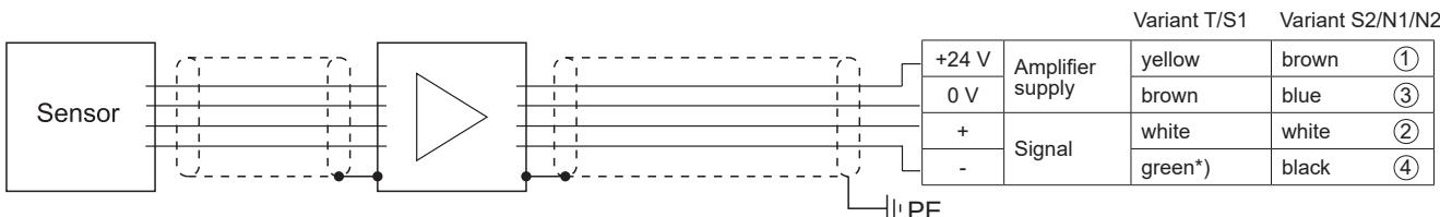
\*) With variant U this line is not in use. The reference potential of the signal is 0 V of the amplifier supply
