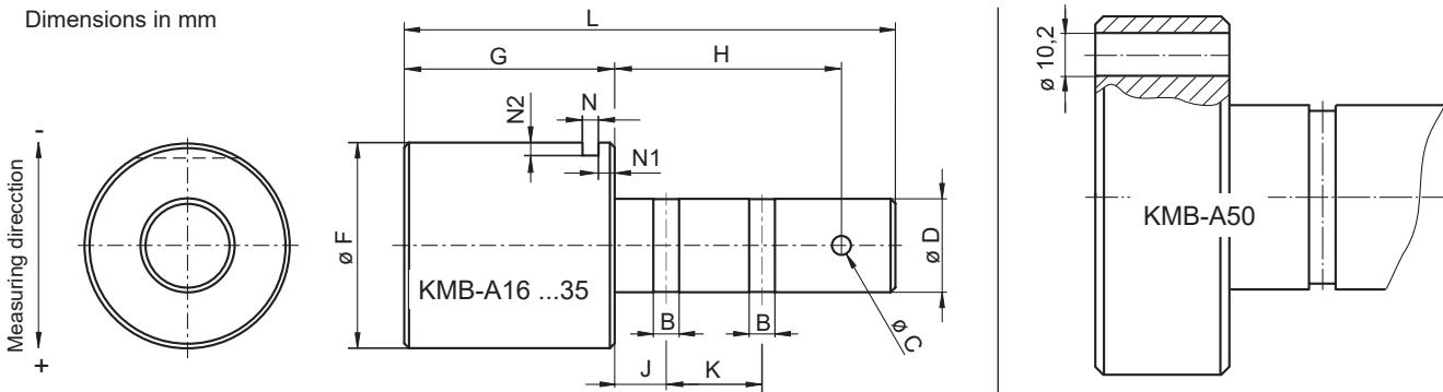
Standard: Calibration in positiv measuring range, KMB12 ...KMB35 are calibrated to tension, KMB50 to compression load
